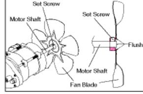
Figure 14. Fan and Setscrew Location.
